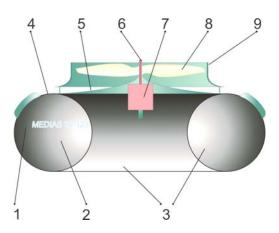
Fig. 11 MEDIAS components [10] 1 - curved upper surface; 2 - steering flaps; 3 - toroidal He chamber; 4 - counter-rotating fins; 5 - inner exhaust profiled cap; 6 - propeller's shaft; 7 - electrical motor and batteries; 8 - propeller; 9 propeller duct
