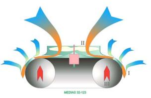
Fig. 12 The sustentation and propulsion components of MEDIAS UAV
