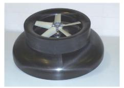
Fig. 14 ODIN – The AESIR's demonstrator for a military Coandă UAV
